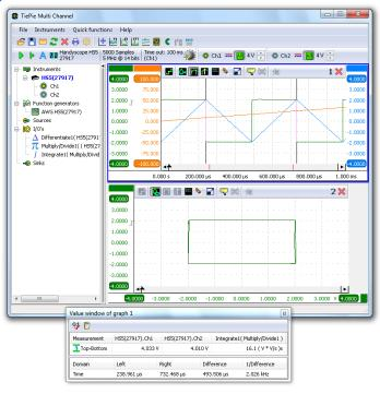
This measurement determines the area of an XY graph, using multiplying, integrating and differentiating I/O's. The area is indicated in the Value window:  $16 V^2$ .
