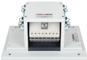
CIP 9138 with PCJ 9202 calibration jig
