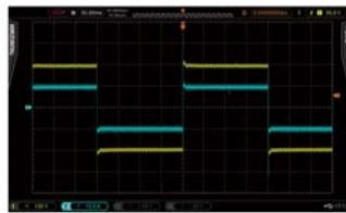
Linear CC mode, PWM 10A 2.5Hz
