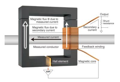
High-frequency currents are detected by the winding (CT), while DC to low-frequency currents are detected by the Hall element.
