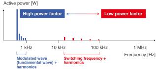
Since the power factor decreases with harmonics, current sensors' phase measurement accuracy becomes key (see right).
