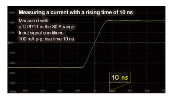
Current probes with a wide frequency band can capture high-speed current fluctuations with a rising time of 10 ns.
