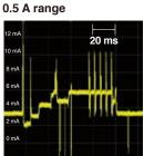
Observing a minuscule current waveform (current consumption of a power-saving device)
