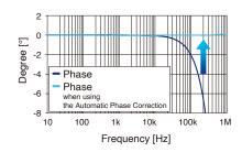
Example of the Automatic Phase Correction for the CT6904A AC/DC current sensor
