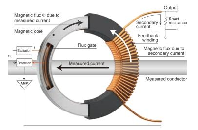
Zero-flux method: achieving stable, wideband measurement from DC to high frequencies
