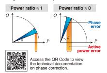
The power factor decreases in the high-frequency range of the switching frequencies and other frequency components. At low power factors, phase error has a significant effect on power measured values.
