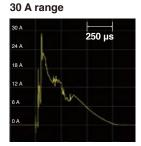
Observing a large current waveform (inrush current)
